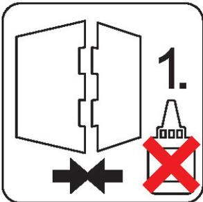
Always dry-fit the parts together without any glue to make sure you are assembling the correct parts.
