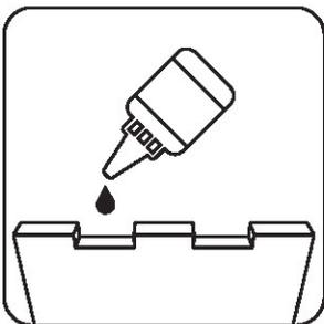
Use a drop of glue along the joints and hold it in place until the glue has sufficiently dried.
