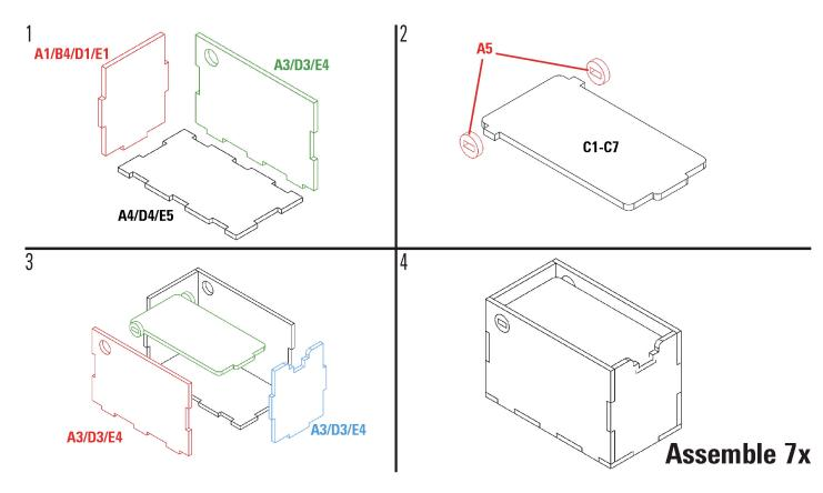
Required parts: A1x2,A2x2,A3x8,A4x4,B1,B4,C1,C2,C3,C4,C5,C6,C7,D1,D2,D3x4,D4x2,E1x3,E3x3,E4x2,E5
