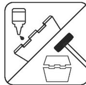
Use a drop of glue along the joints and press the parts together or use a hobby hammer with slight force for assembly.
